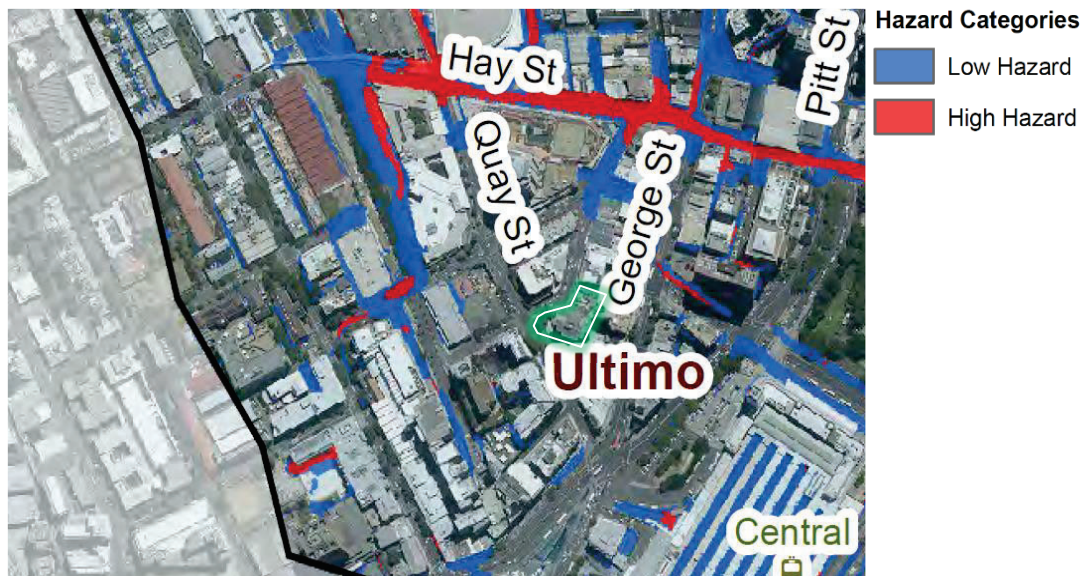
Figure 8 - 187 Thomas Street location with respect to available 1% AEP event flood hazard mapping (source: Darling Harbour Catchment Floodplain Risk Management Study)
